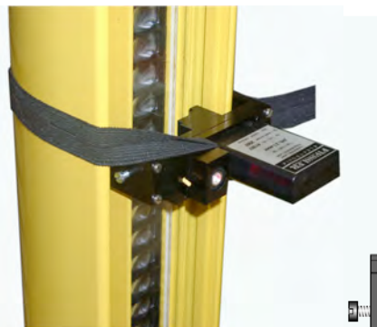
Column mounting mount the elastic band only on one screw
